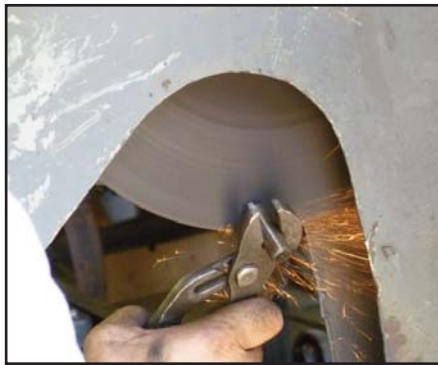
Fig. 11 Chamfering a new cylindrical bearing on a chop saw.
