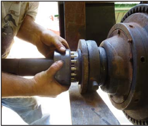
Fig. 21 Bearing cage sleeve being placed over cylindrical roller bearing cage.
