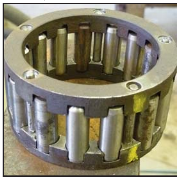
Figs. 14-17 (left to right): New (& old) cylindrical bearings and pins in place in one-half of cage; Both halves of cage in place with pins to be peened over; Louis peening over pins; Completed cylindrical roller bearing cage.
