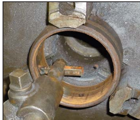
Figs. 18-19 (left & center): Roller bearing cage sleeve being turned on metal lathe. Fig. 20 Finished cage sleeve with new grease fitting (sticking out on left).
