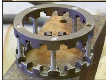
Fig. 13 Cage assembly with new pins (minus the cylindrical bearings).
