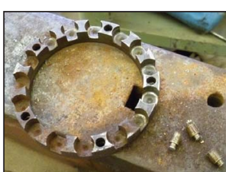
Fig. 8 One half of roller bearing cage with heads of pins removed.
