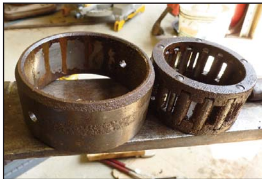
Fig. 5 Rusted and seized cylindrical roller bearing cage and sleeve (left).
