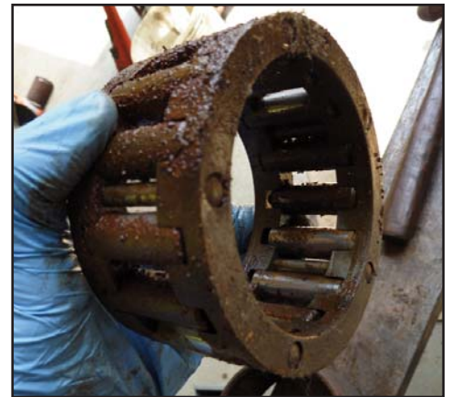
Fig. 6 Close-up of seized cylindrical roller bearing cage.
