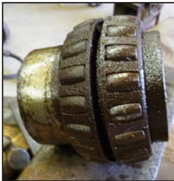
Fig. 4 Seized double-row tapered roller bearing.
