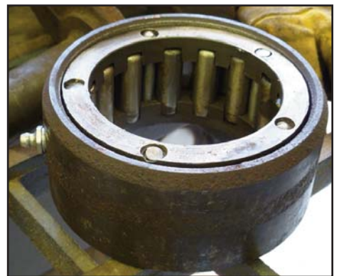
Figs. 18-19 (left & center): Roller bearing cage sleeve being turned on metal lathe. Fig. 20 Finished cage sleeve with new grease fitting (sticking out on left).
