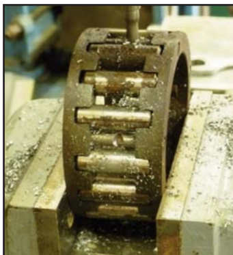
Fig. 7 Drilling out pins.
