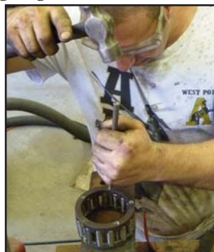
Figs. 14-17 (left to right): New (& old) cylindrical bearings and pins in place in one-half of cage; Both halves of cage in place with pins to be peened over; Louis peening over pins; Completed cylindrical roller bearing cage.
