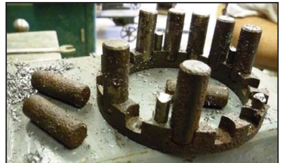
Fig. 9 Opened cylindrical roller bearing cage with rusted and pitted bearings.
