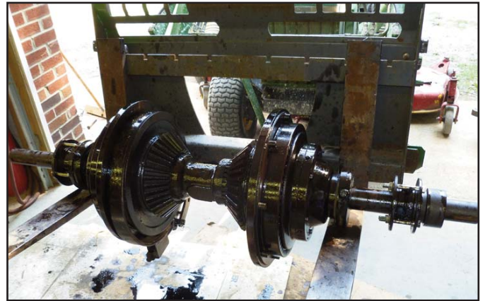
Fig. 24 (left): Lubricating the main gear shaft through a new grease fitting. Fig. 25 (right): Main gear shaft coated with "special" mixture.
