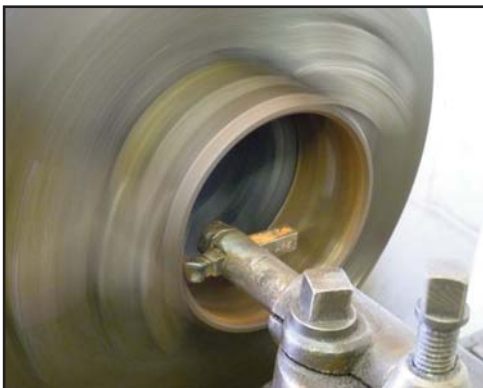
Figs. 18-19 (left & center): Roller bearing cage sleeve being turned on metal lathe. Fig. 20 Finished cage sleeve with new grease fitting (sticking out on left).
