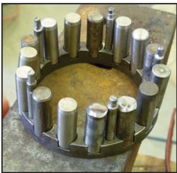
Figs. 14-17 (left to right): New (& old) cylindrical bearings and pins in place in one-half of cage; Both halves of cage in place with pins to be peened over; Louis peening over pins; Completed cylindrical roller bearing cage.
