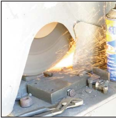
Fig. 10 Cutting a new cylindrical bearing on a chop saw.
