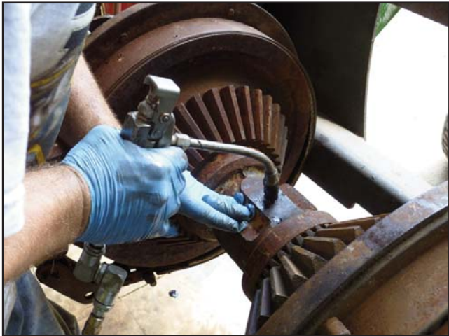
Fig. 24 (left): Lubricating the main gear shaft through a new grease fitting. Fig. 25 (right): Main gear shaft coated with "special" mixture.
