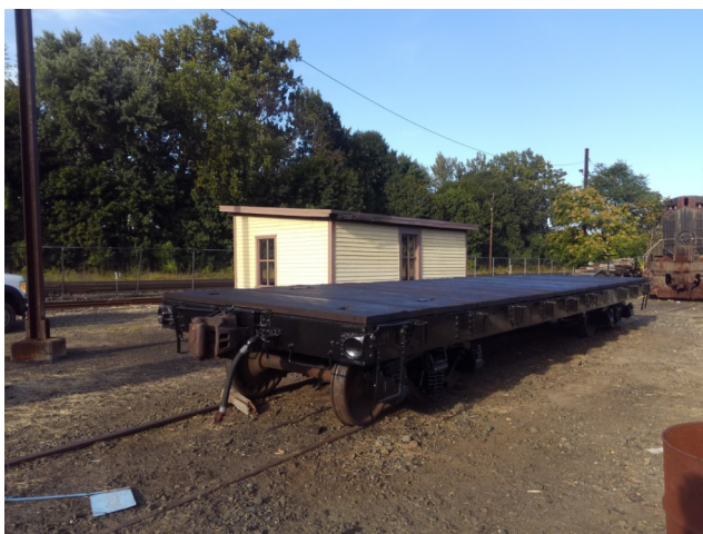
Left: A southeast facing view of the redecked and repainted X-578. Photo by Justin Chapin.
